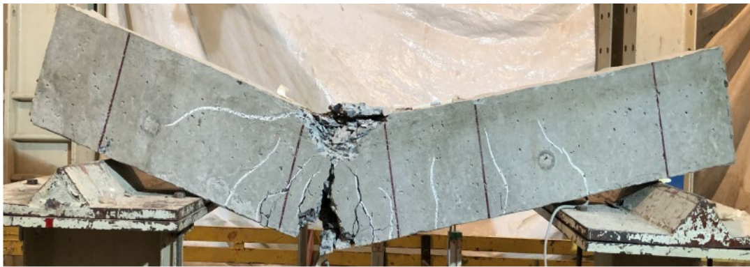
Fig. 15 Crack pattern in ordinary prestressed reinforced concrete (OPRC) beam
