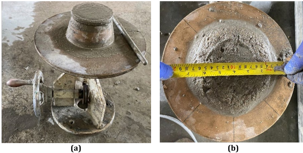
Fig. 4 (a) Flow table test equipment (b) Testing in progress
