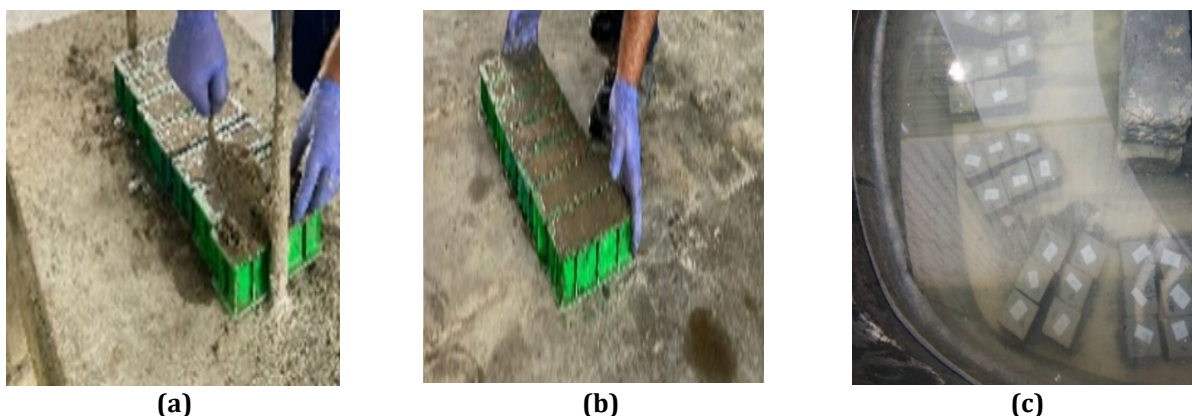
Fig. 3 Mortar cubes preparation work
