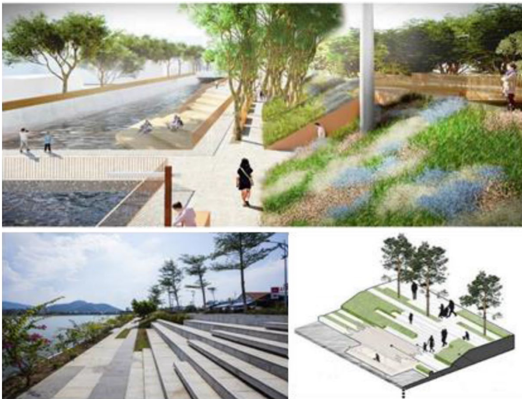
Fig. 13 Maximize the design of soft embankment and green embankment landscape (3 - Buffer and vegetated filter strips) close to the water surface in the middle of the river. (Source [3])
