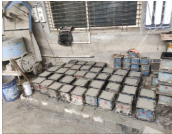
Fig. 4 Casting of concrete cubes
