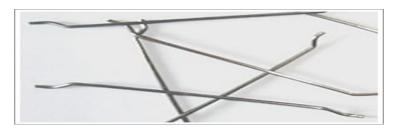
Figure 1: Hooked-end shape steel fibers used in this Study
