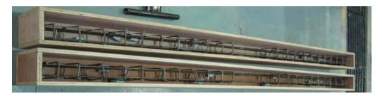
Figure 2: Appearance of the RC and the SFARC beams before casting
