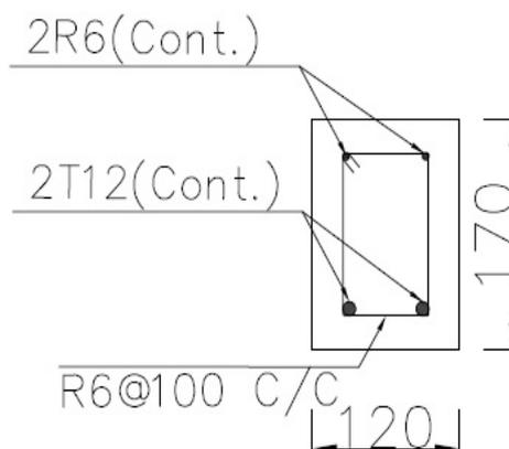
**Figure 3:** Cross Section of the RC and the SFARC Beams (dimensions in mm)
