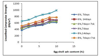
Figure 5: Variations of Unconfined Compressive Strength with Egg Shell Ash
