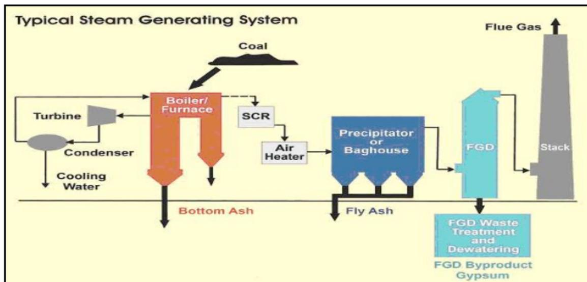
**Figure 1:** Typical thermal power plant & resulting waste generated
