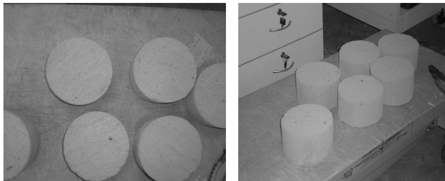
Figure 2. Foamed concrete sample
