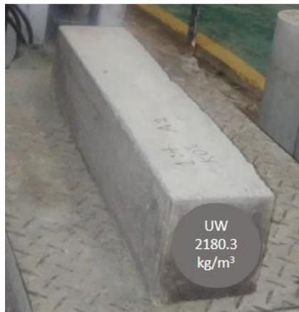
**Fig. 13 - Mortar beam specimen**
