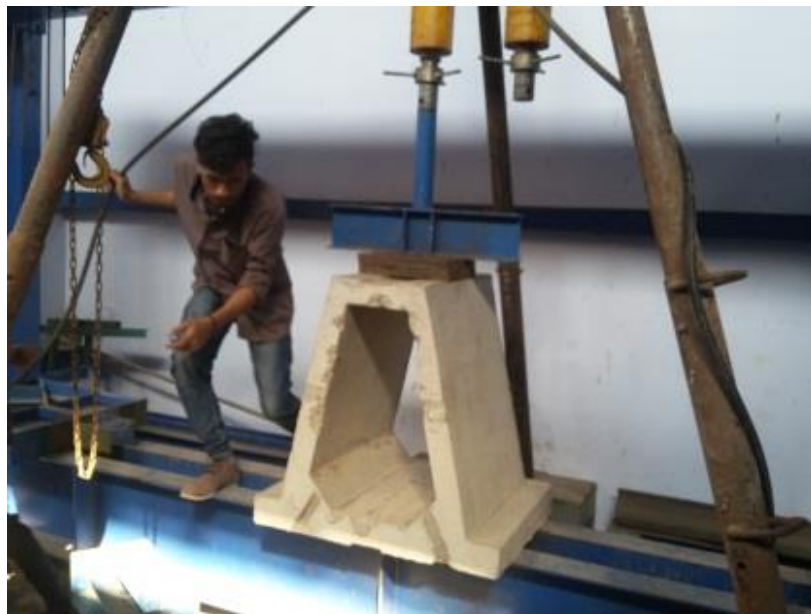
Fig. 3 - Compression and Flexural test specimens.
