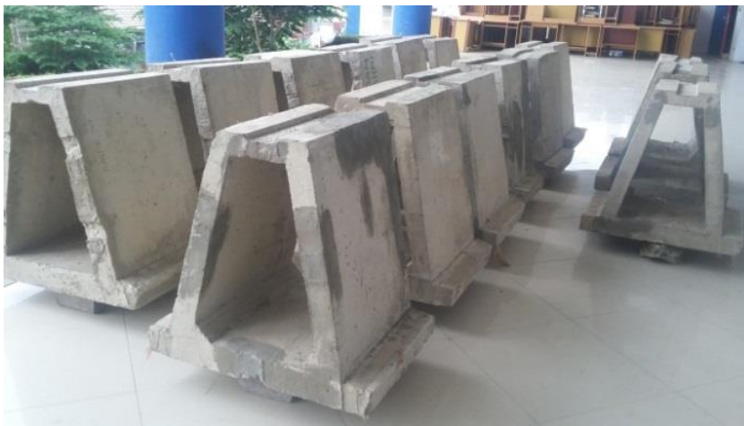
Fig. 2 - Precast foundation specimens.
