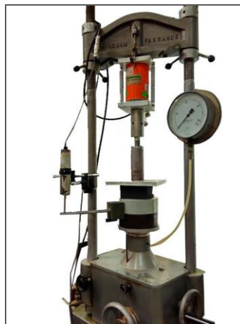
Fig. 3 - Compression test set up (Preliminary test).
