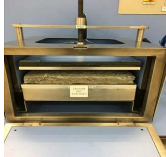
Fig. 11 - Thermal Conductivity Test
