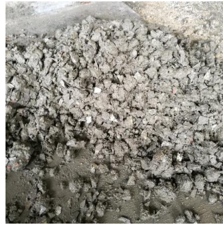
Fig. 8 - Completely Mixed Concrete
