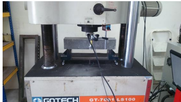
Fig. 4-Flexural strength test setting up with 3-point load
