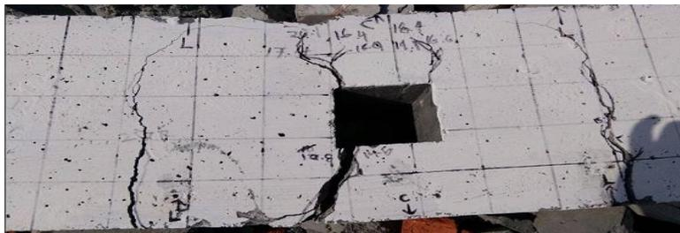
**Fig. 11 - Failure mode of unstrengthened concrete beams with square opening, Beam BSO.**
