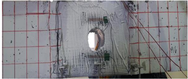
**Fig. 4 - Strengthening configuration with TRC wrap.**
