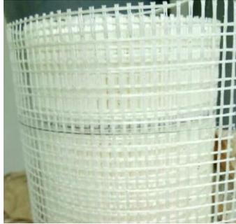
**Fig. 1 - Textile Reinforced Concrete (TRC) wrap.**
