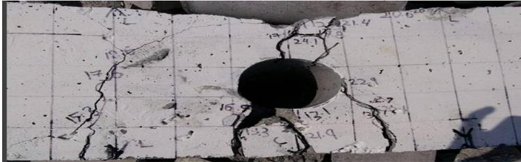
**Fig. 10 - Failure mode of unstrengthened concrete beams with circular opening, Beam BCO.**
