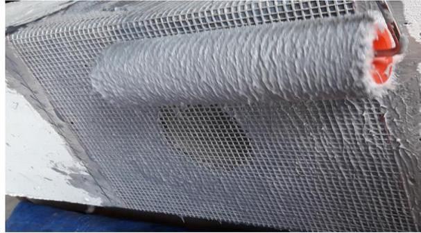
**Fig. 3 - Strengthening configuration with TRC wrap.**
