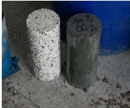
**Figure 1:** Concrete cylinder immersed in 5% H<sub>2</sub>SO<sub>4</sub> for 28 days (Left)
