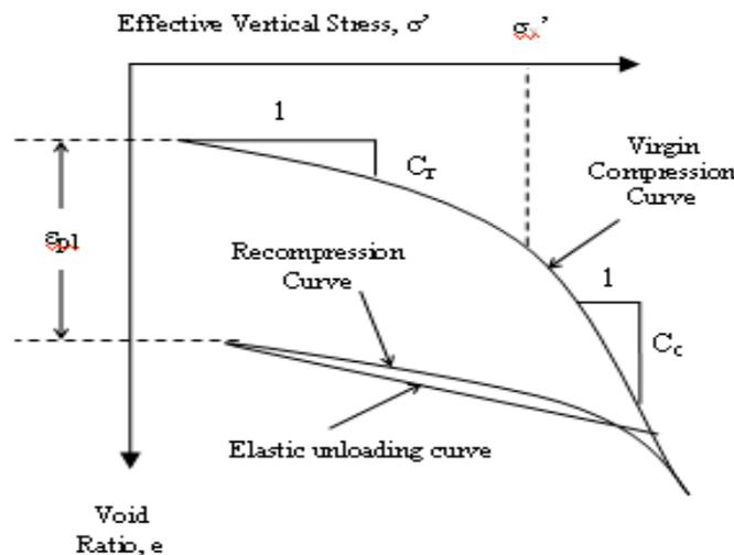
Figure 2. Typical e-log  $\sigma'$  curve
