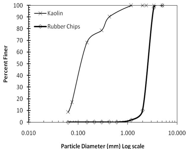
Figure 1. Grain size distribution of kaolin and rubber chips
