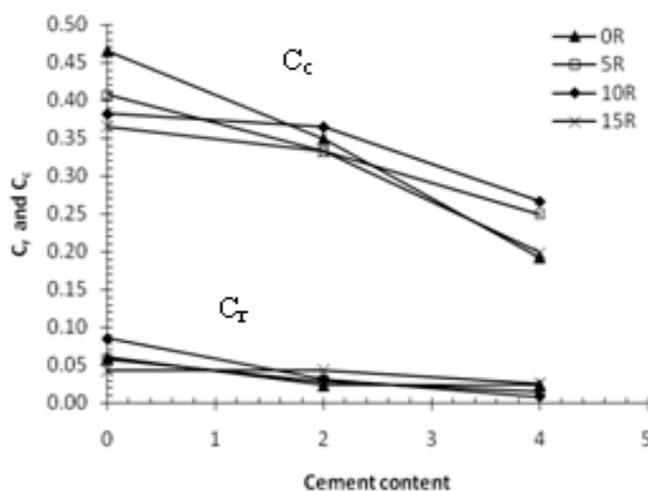
Figure 12. Effect of cement-rubber chips on the compression and rebound indices  $C_c$  and  $C_r$
