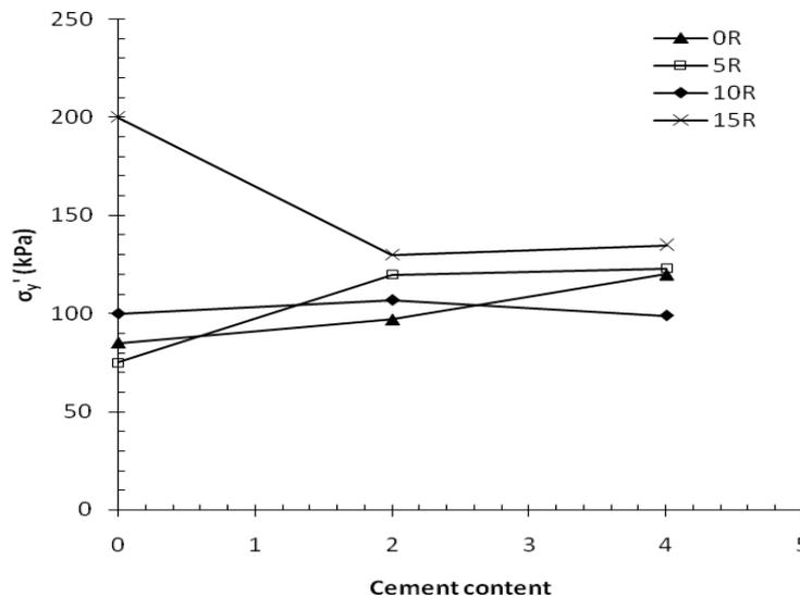
Figure 11. Effect of cement-rubber chips on the vertical effective yield stress
