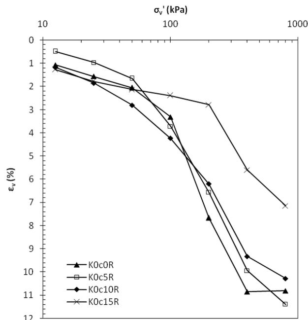
Figure 3. Compression curve for 0c
