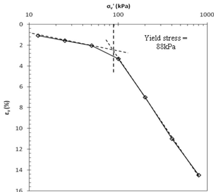
Figure 6. Illustration of effective vertical stress determination
