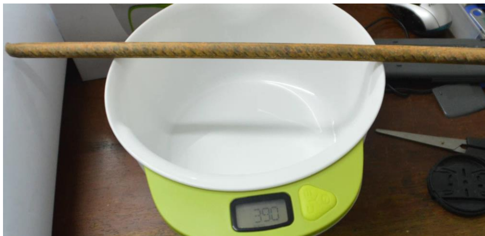
Fig. 2 - Carrying Measurements with Samples taken from the Failed Retaining Wall
