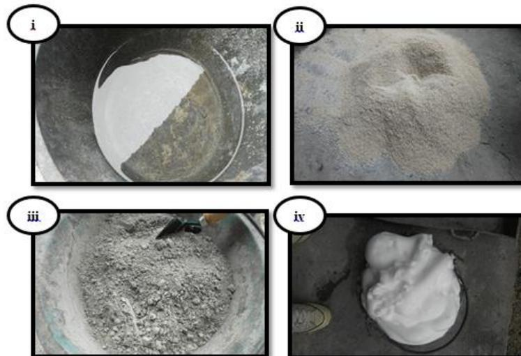
**Fig. 2 - Materials of foam concrete; (i) sand, (ii) Ordinary Portland Cement (OPC), (iii) water and (iv) micro bubbles foaming**
