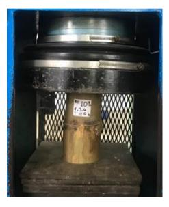
Fig. 4 - Set up for Compression Test
