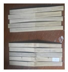
Fig. 17 - Failure pattern of bending test specimen
