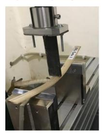
Fig. 10 - Set up for Bending Test
