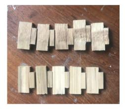
Fig. 15 - Failure pattern of shear test specimen
