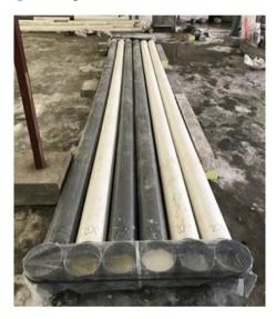
Fig. 2 - Bamboo soaking process
