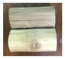
Fig. 11 - Failure pattern of compressive test specimen
