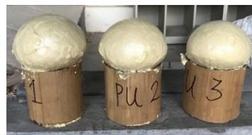
**Fig. 3 - Bamboo specimens filled with Polyurethane Foams (PU)**
