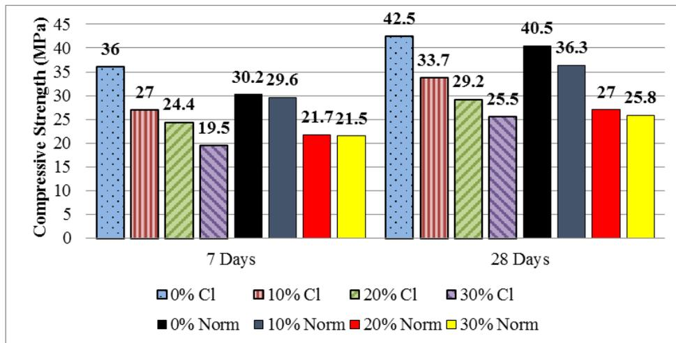
Fig. 6 - Compressive strength of concrete for both exposures
