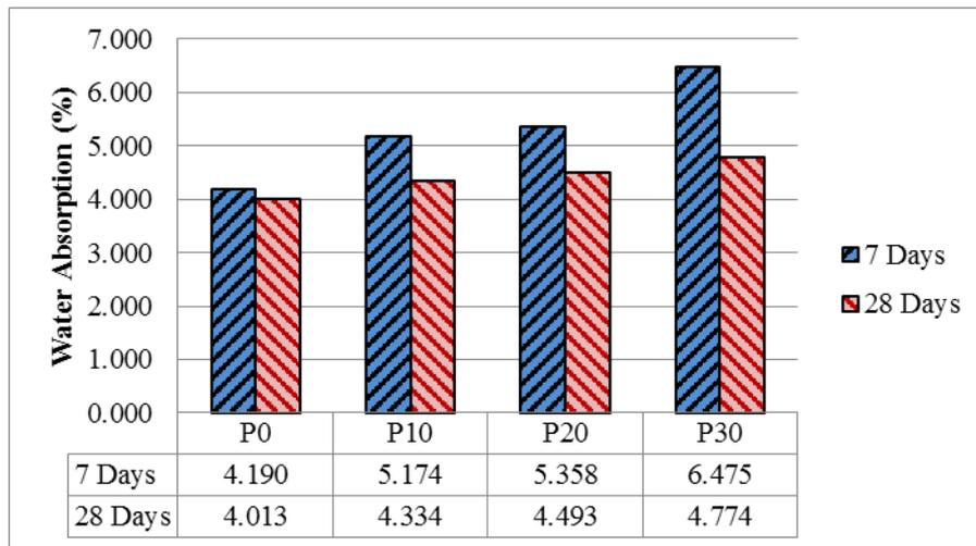
**Fig. 9 - Water absorption in 7 and 28 days in chloride**
