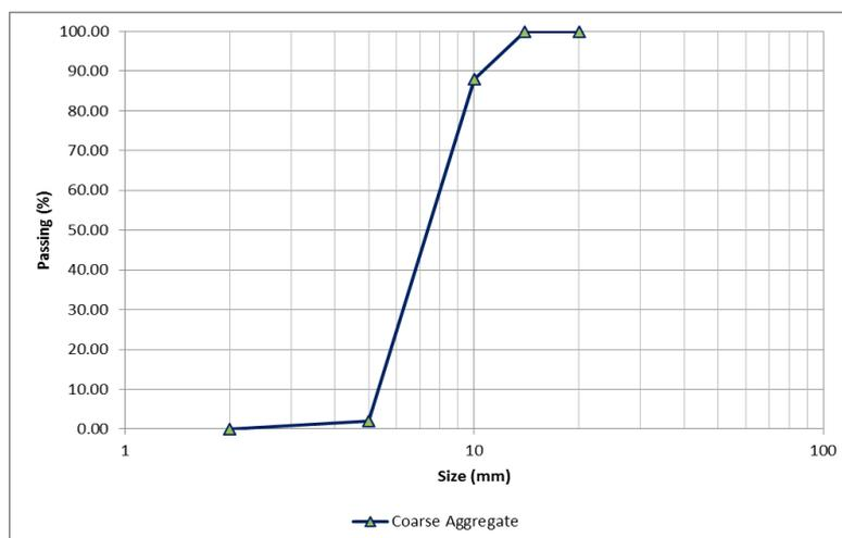
**Fig. 2 - Sieve analysis of coarse aggregate**
