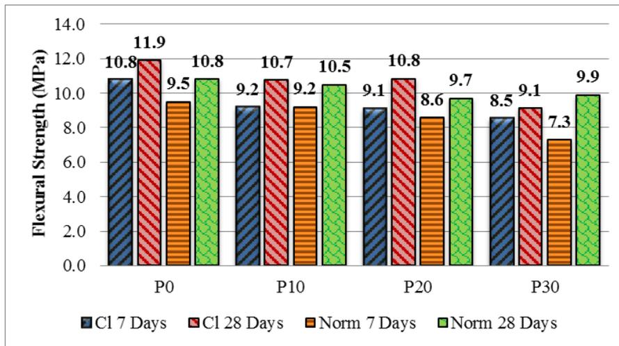
Fig. 7 - Flexural strength of concrete in both exposures
