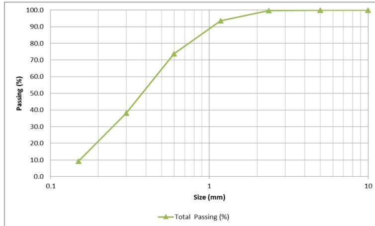
Fig. 3 - Sieve analysis of fine aggregate
