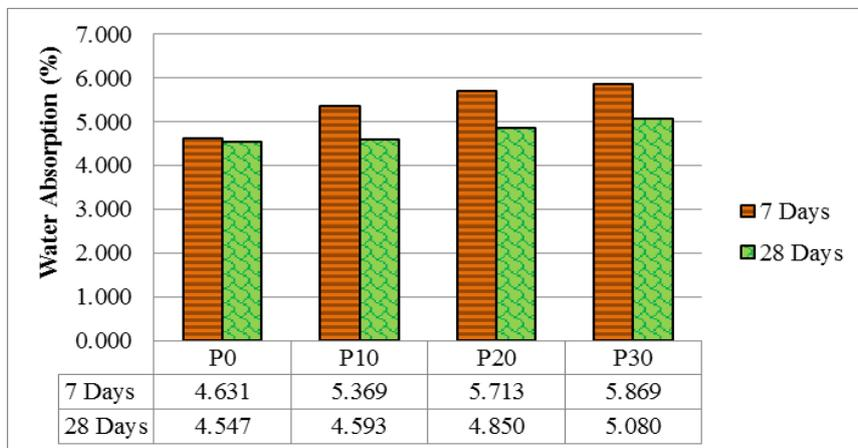
Fig. 8 - Water absorption in 7 and 28 days in the water
