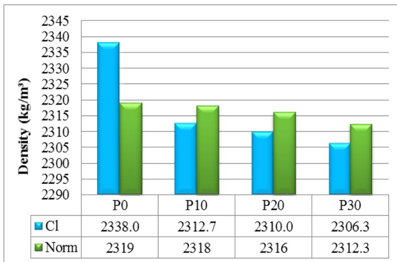
Fig. 5 - Density of concrete for both exposures
