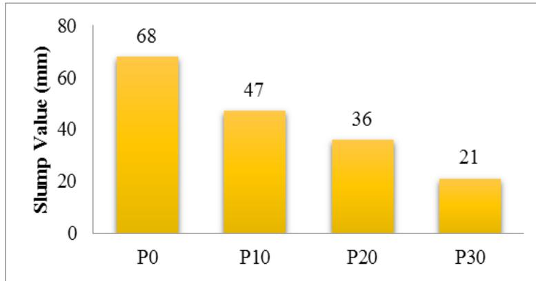
Fig. 4 - Workability of concrete containing POFA
