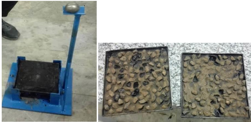
Fig. 1 - Vialit test apparatus and Samples prepared for vialit test
