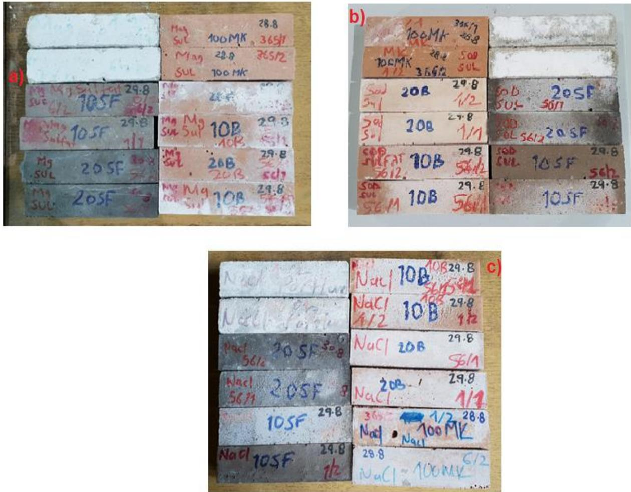
**Fig. 11 - Visual inspection in all samples over 12 months a) with magnesium sulfate effect b) with sodium sulfate effect c) with sodium chloride effect**
