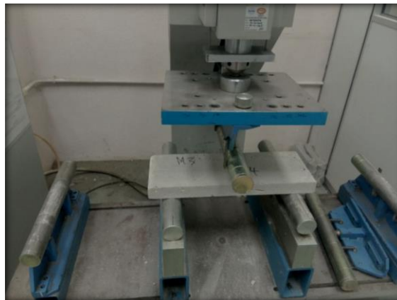
Fig. 8 - The flexural test was performed according to ASTM C293
