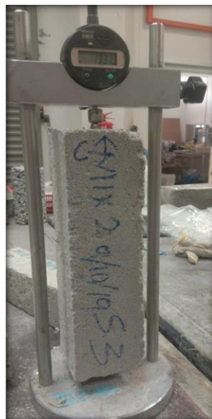
Fig. 12 - Shrinkage test was carried out according to ASTM: C 878
