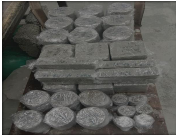
Fig. 6 - All specimens were wrapped with a plastic sheet before the testing day
