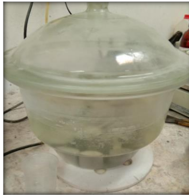
Fig. 11- Porosity test was performed according to BS 1881: Part 122
