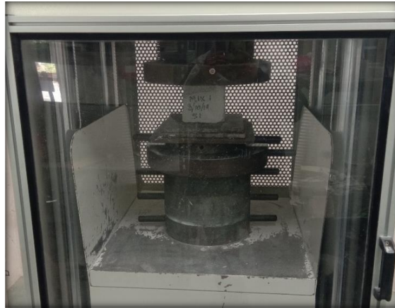
Fig. 7 - Compression Test according to BS EN 12390: Part 3
