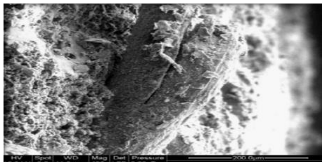
Fig. 29 - Surface debonding between OPT fibre and cement matrix
