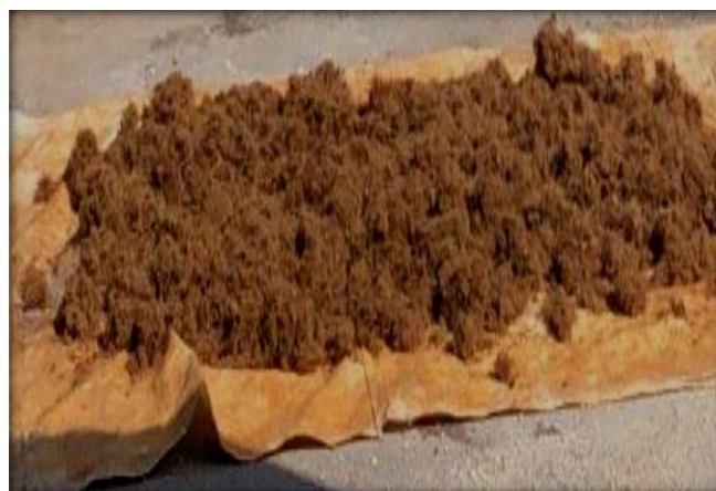
Fig. 3 - Oil palm trunk fibre was dried for two days
