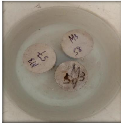
Fig. 10 - Water absorption test was performed according to BS 1881: Part 122
