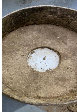
Fig. 4 - The sample shape after 10cm penetration for unsoaked California bearing ratio
