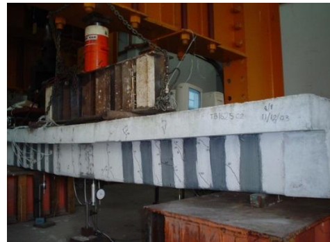
(b) CFF repaired beam -TS1-1
