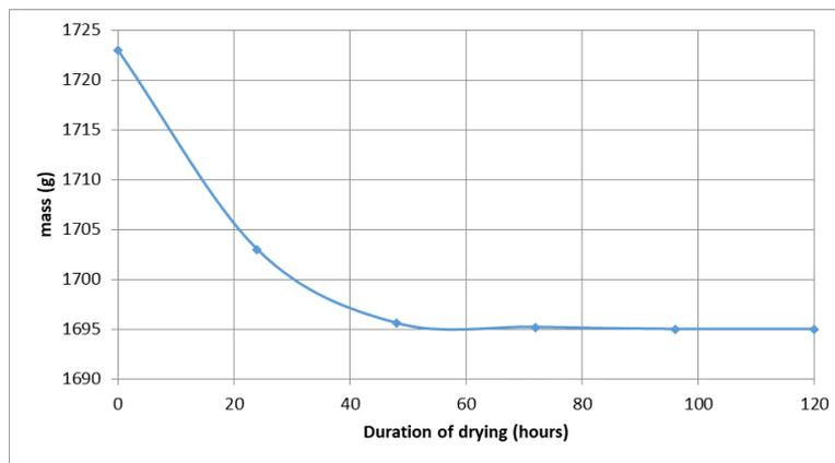
**Fig. 11 - Curve of variation of the mass of the dry bricks as a function of time**
