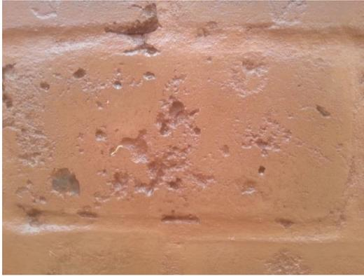
**Fig. 13 - Quite marked effect of decrepitude of the wall (dosage of 5 and 6%)**
