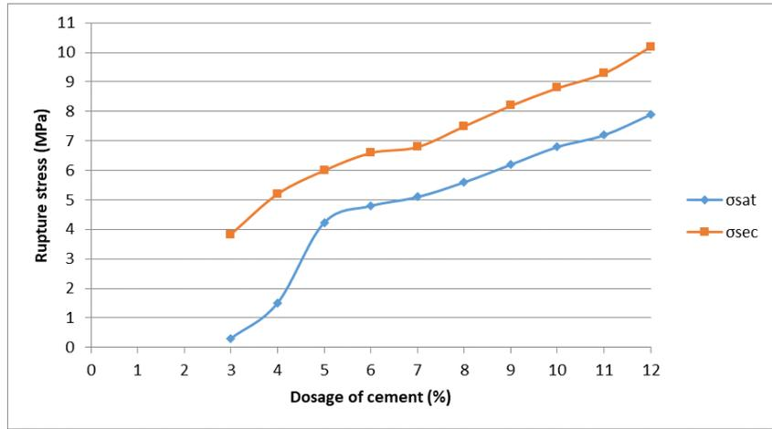
Fig. 16 - Variation of the  $\sigma_{sat}$  and  $\sigma_{dry}$  as a function of dosage of cement
