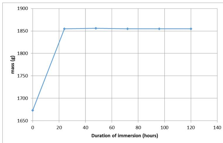
Fig. 10 - Curve of variation of the mass of the immersed bricks as a function of time
