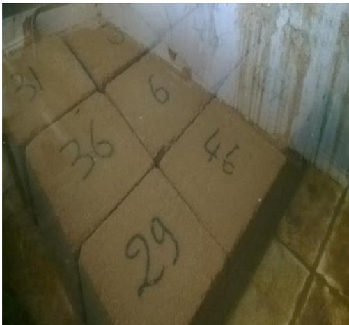
Fig. 7 - Immersion of the bricks
