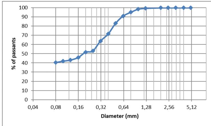
Fig. 9 - Granulometric curve of the soil
