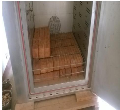
Fig. 8 - Drying of the bricks
