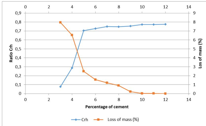
Fig. 17 - Variation of  $C_{rh}$  and loss of mass as a function of dosage of cement
