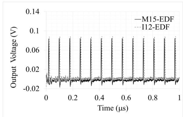
**Fig. 4** The repetition rate of the Mode-Locked fiber laser by using M15, and I12-EDF.
