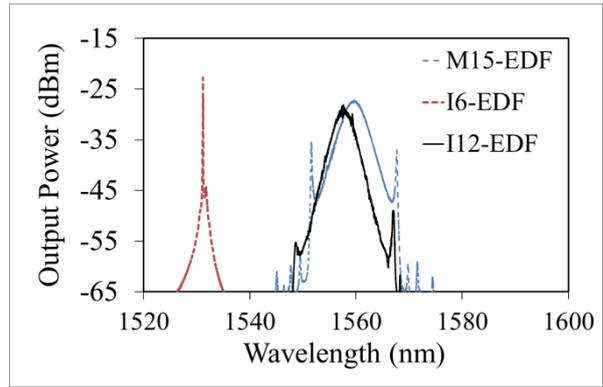
**Fig. 3** The Output spectra for Passively Mode-Locked fiber laser by using M15, I6 and I12-EDF.
