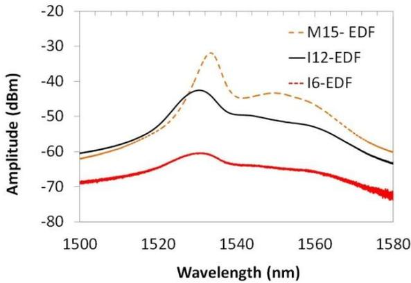
**Fig. 2** Optical output spectra of the amplified spontaneous emission (ASE) for three different fibers.
