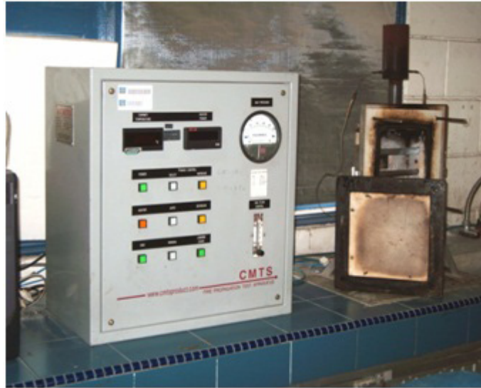
Diagram 1 A fire-propagation apparatus at SIRIM
