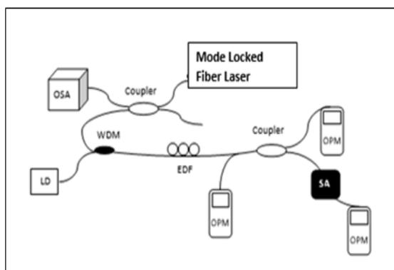
**Fig. 5** Schematic diagram of the absorption measurement of Pt as SA.
