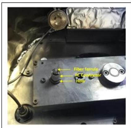
**Fig. 1** The image of the FC connector inside the sputtering machine (rewritten as fiber ferrule, FC connector and hole), DC Sputter QT300T D by Quorum Technologies.
