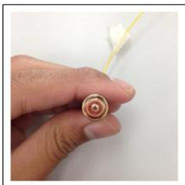
**Fig. 2** The coated 10 nm of Pt on fiber ferrule by using DC Sputter QT300T D by Quorum Technologies.
