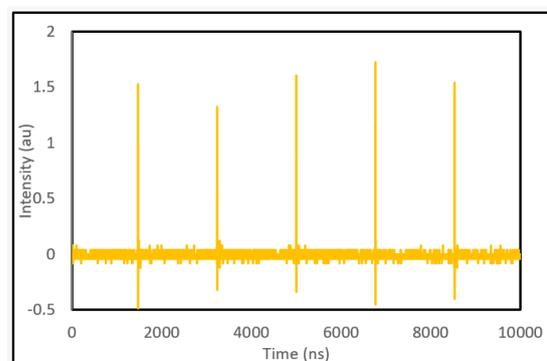
**Fig. 7** Repetition rate of the Q-switched pulses for 600 mA.
