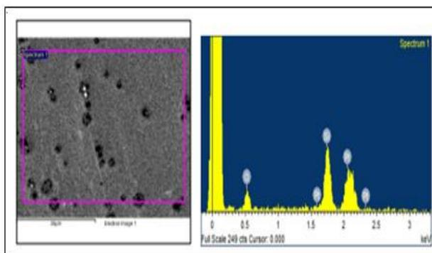
**Fig. 4** EDX spectrums for deposited Pt.
