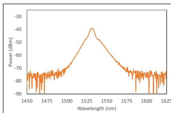
**Fig. 6** Q-switched spectrum at 600 mA.
