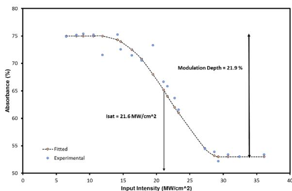
**Fig. 8** The transmission spectrum of Pt with a modulation depth of 21.9%.
