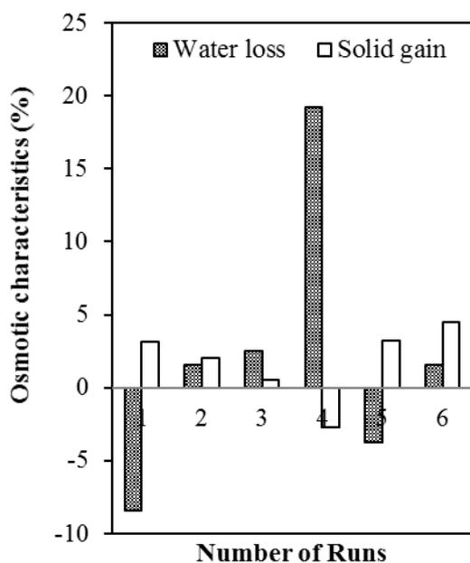
**Fig. 1** Water loss and solid gain as osmotic characteristics that correspond to the number of runs.
