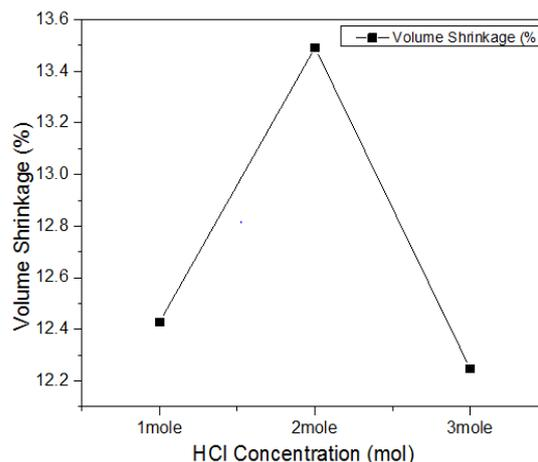
**Fig. 3** Variation of Volume Shrinkage versus HCl concentration.
