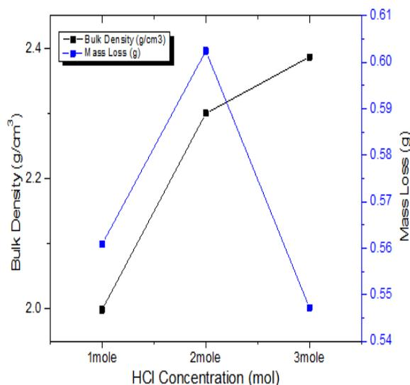
**Fig. 2** Variation Bulk Density and Mass Loss versus HCl concentration.
