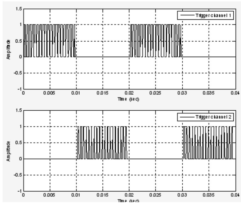
**Figure 18:** Simulated SPWM trigger signal in two channels in SIMULINK
