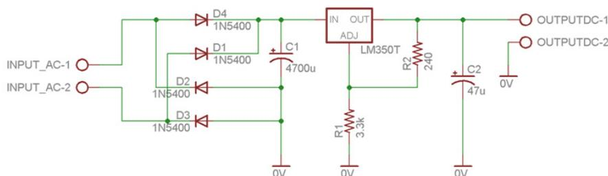
Figure 6: Bridge rectifier circuit
