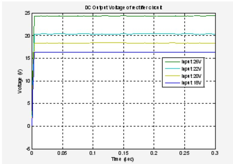
Figure 13: Simulated output of rectifier circuit.
