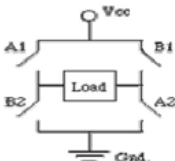
**Figure 3:** Standard H-Bridge circuit
