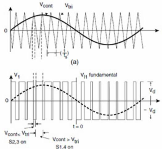
**Figure 4:** SPWM trigger signal generation method through bipolar switching. (a) Reference sine signal is compared with carrier sawtooth signal (b) Generated SPWM trigger signal
