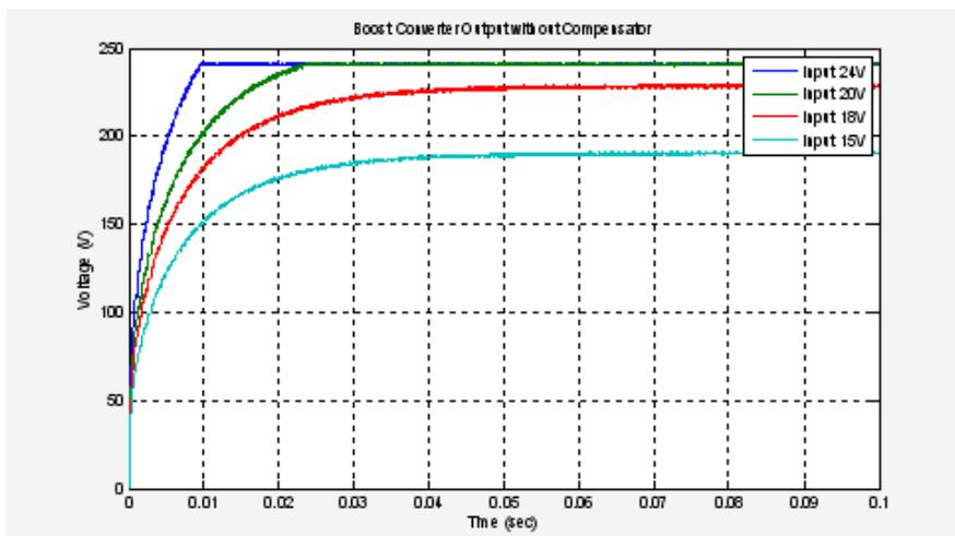
Figure 14: Simulated output of Boost DC-DC Converter
