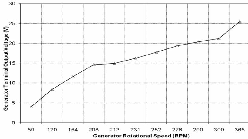
**Figure 12:** 500W Voltage generated at terminal of wind generator simulator rotated at different speed.
