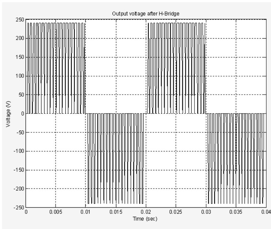
**Figure 19:** Simulated output voltage of H-bridge ci
