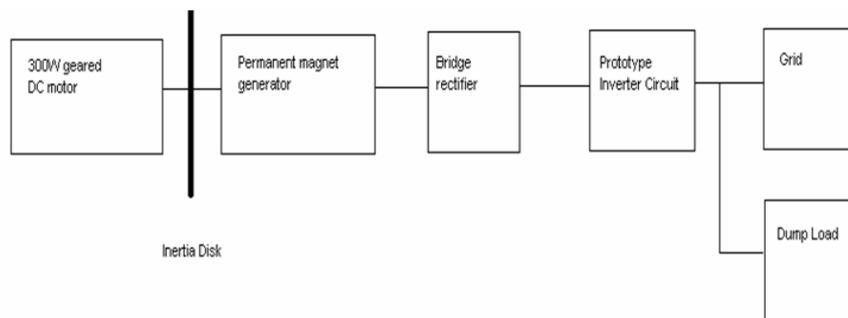
**Figure 9:** Proposed Lab-scale experimental rig
