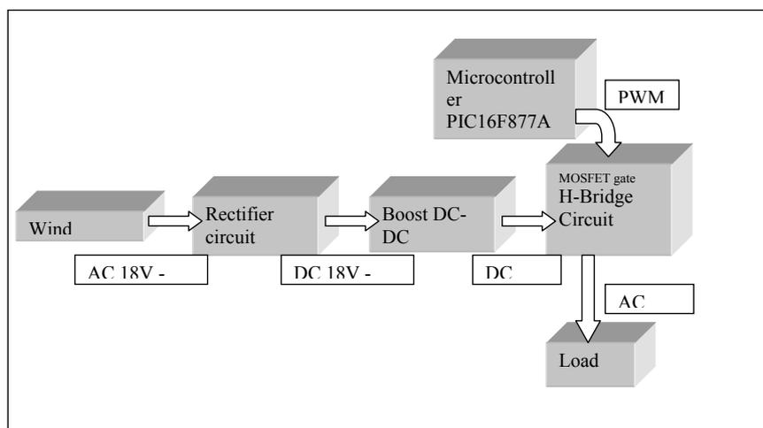
Figure 5: Block diagram of proposed system
