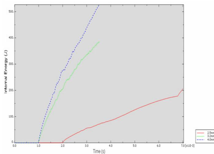
**Figure 7:** Energy absorbed for various wall thickness at constant speed 30m/s
