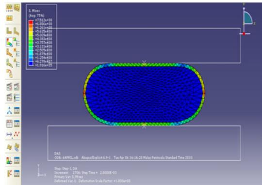
**Figure 3:** Collapse pattern of foam-filled Tube
