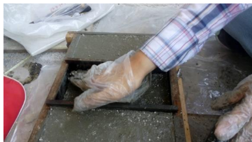
Fig. 4 Compacting the mortar inside the mould using hand tamping
