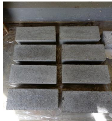
Fig. 6 Demoulded brick in curing period before testing day.
