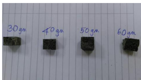
Fig. 2 Dice size samples for SEM test
