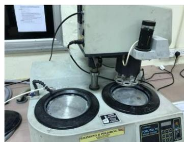
**Fig. 3** Modified Grinder Machine Metkon, Turkey
