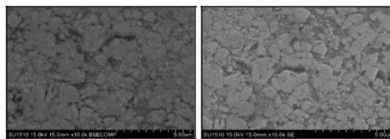
**Fig. 5** Surface Morphology for HVOF Coating with 30LPM Oxygen Flowrate. Image (Left) and SE Image (Right)
