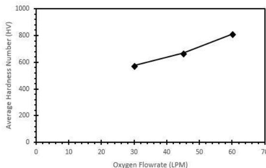
**Fig. 9** Average Vickers Hardness Graph
