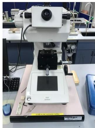
**Fig. 2** Vickers Micro-Hardness Tester Shimadzu, Japan
