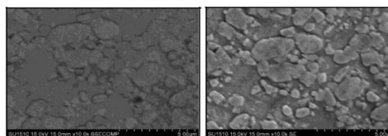
**Fig. 6** Surface Morphology for HVOF Coating with 45LPM Oxygen Flowrate. BSE Image (Left) and SE Image (Right)
