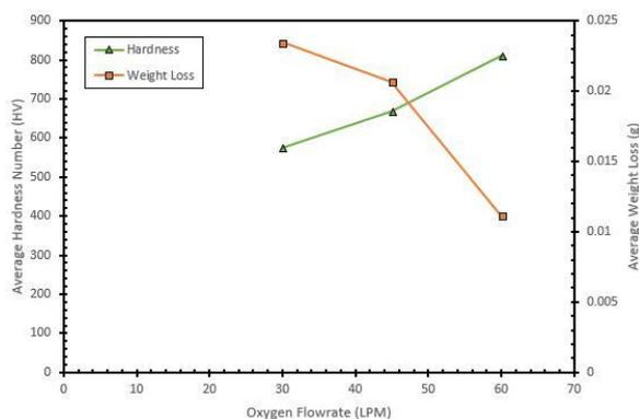
**Fig. 10** Average Weight Loss of Three Different Parameters of HVOF Coating
