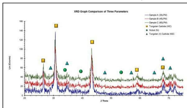
**Fig. 8** Combined XRD Analysis of Three Different Parameters of HVOF Coating
