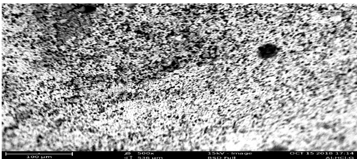
Fig. 7 - Micrograph of aluminum in 1.4 M HCl solution with 0.1 M glutaraldehyde.
