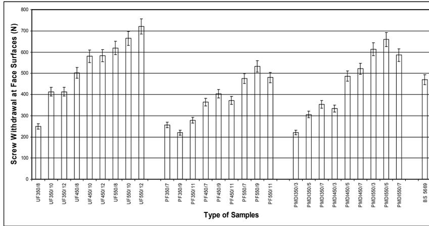
Figure 10: The screw withdrawal (face section) results of kenaf particleboards
