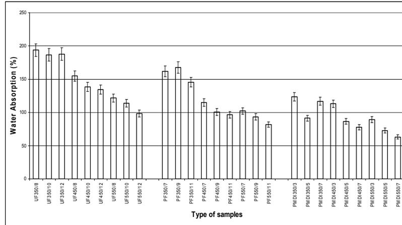
**Figure 13:** The water absorption results of kenaf particleboards
