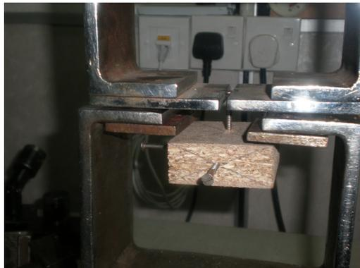
**Figure 9:** The screw withdrawal test
