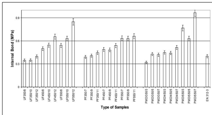
Figure 8 : The IB results of kenaf particleboards
