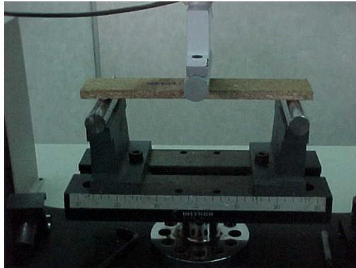
**Figure 4:** Bending strength test
