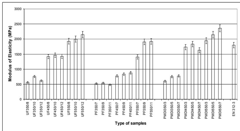
**Figure 6:** The MOE results of kenaf particleboards
