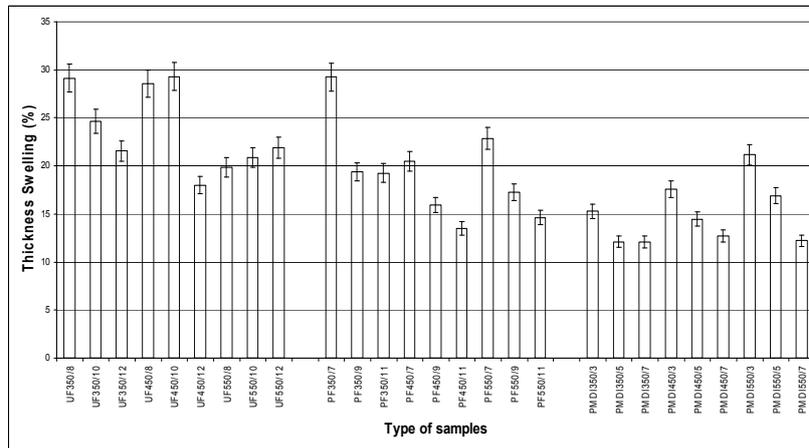
**Figure 14:** The thickness swelling results of kenaf particleboards
