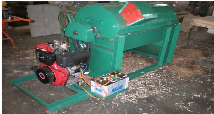
**Figure 1:** The kenaf decorticating machine
