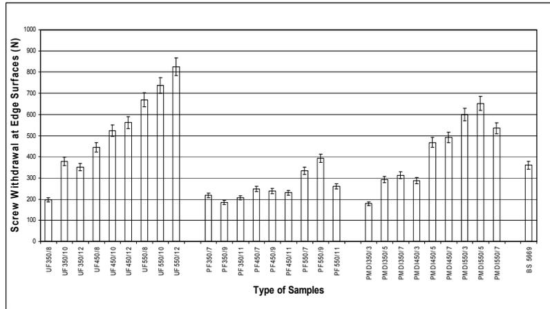
Figure 11: The screw withdrawal (edge section) results of kenaf particleboards
