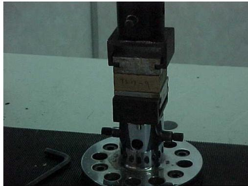
Figure 7: Internal bond test
