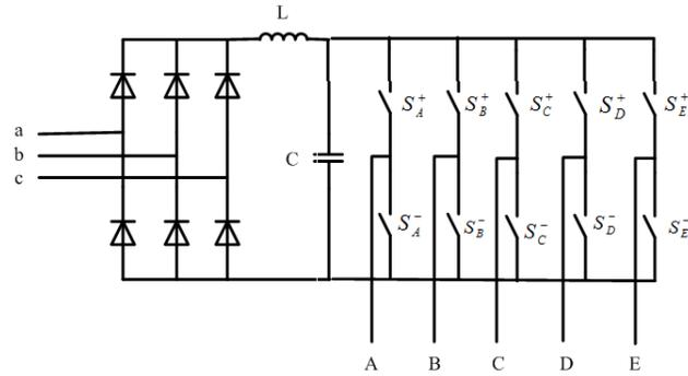
**Figure 1:** Five-phase voltage source inverter
