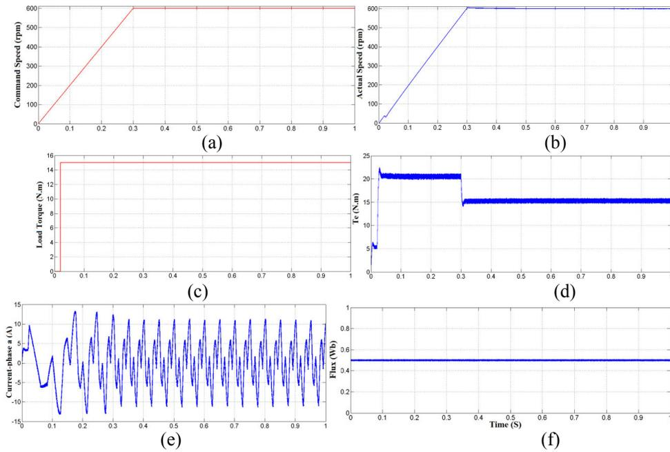
**Figure14:** Simulation of classical DTC, (a) command speed, (b) actual speed, (c) load torque, (d) electromagnetic torque, (e) stator current (phase-a), (f) stator flux
