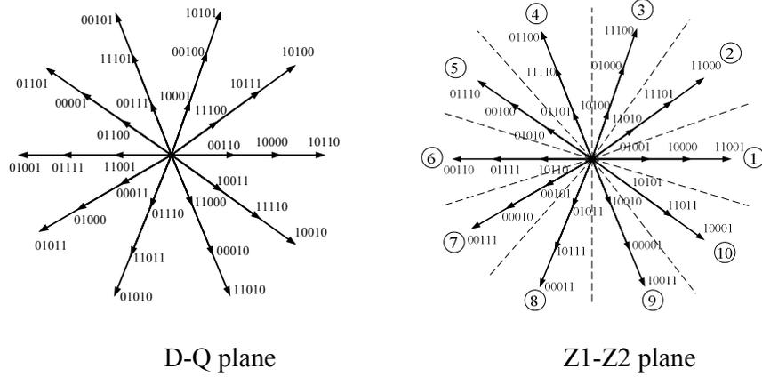
**Figure 3:** Thirty two voltage vectors of a five-phase VSI in D-Q and Z1-Z2 subspaces
