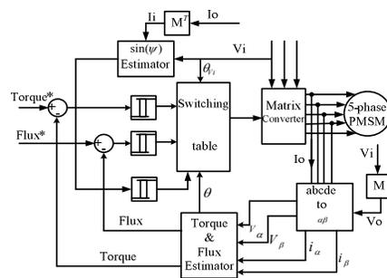
**Figure 10:** Schematic diagram of proposed DTC using matrix converter
