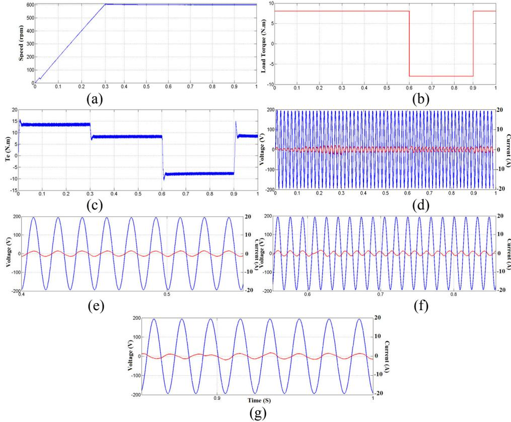
**Figure 17:** Simulation of proposed DTC, (a) actual speed, (b) load torque, (c) electromagnetic torque, (d) filtered input line current and its corresponding voltage (phase-a), (e) filtered input line current from Sec. 0.4 to 0.55, (f) filtered input line current from Sec. 0.55 to 0.85, (g) filtered input line current from Sec. 0.85 to 1
