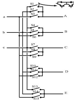
**Figure 6:** Schematic diagram of a three-phase to five-phase matrix converter
