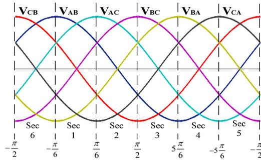
**Figure 9:** Six sectors of input voltage vectors
