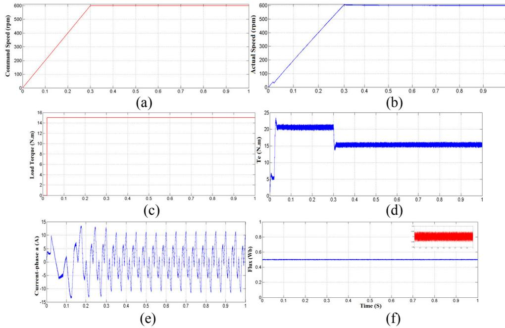
**Figure 15:** Simulation of proposed DTC, (a) command speed, (b) actual speed, (c) load torque, (d) electromagnetic torque, (e) stator current (phase-a), (f) stator flux
