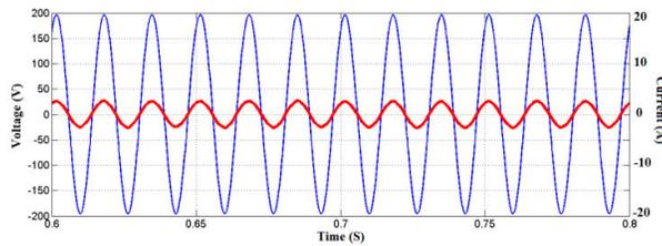
**Figure 16:** Filtered input line current and its corresponding voltage (phase-a)
