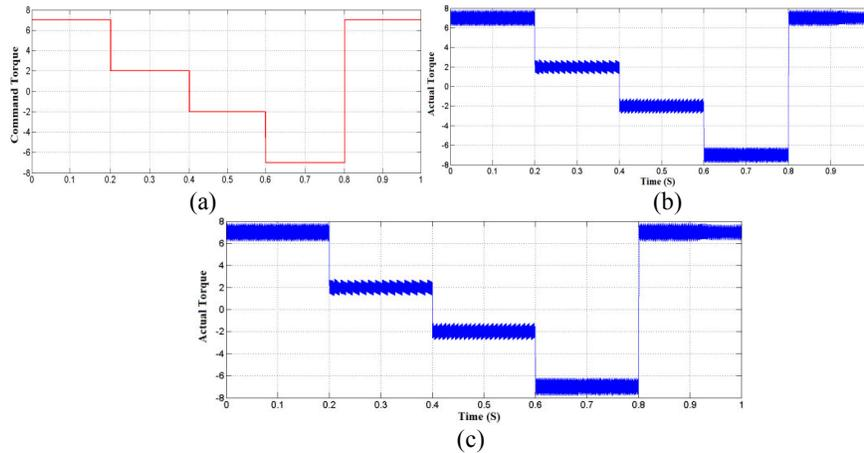
**Figure 11:** From top to bottom: (a) command torque, (b) actual torque for proposed DTC, (c) actual torque for classical DTC
