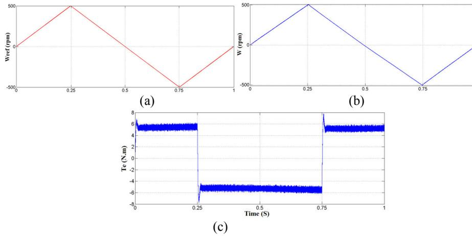
**Figure 13:** (a) command speed, (b) actual speed, (c) electromagnetic torque under no load condition
