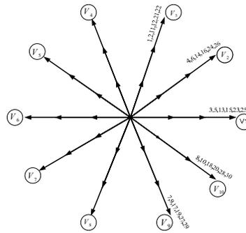
**Figure 7:** Output line-to-neutral voltage vector configurations (large vectors)
