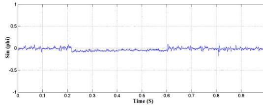
**Figure 12:** Power factor control capability, ( $\sin \phi = 0$ )
