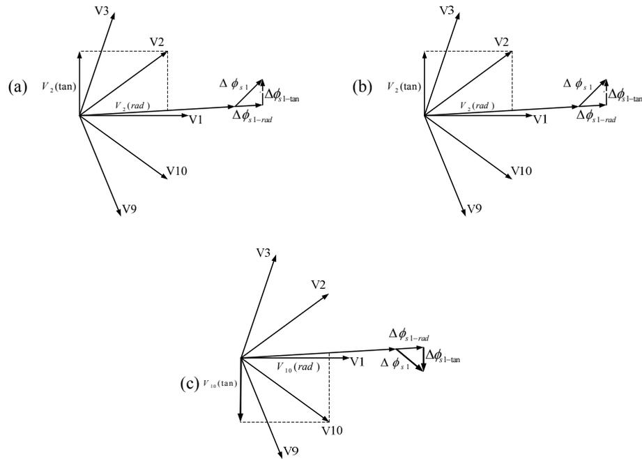
**Figure 4:** Effects of voltage vectors on electromagnetic torque and stator flux magnitude. (a) Effects of voltage vector  $V_2$ , (b) Effects of voltage vector  $V_3$ , (c) Effects of voltage vector  $V_{10}$
