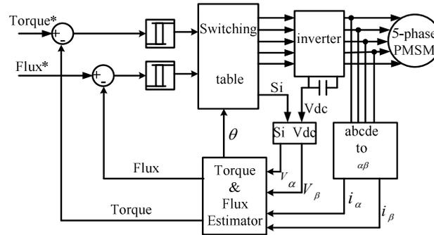
**Figure 5:** DTC of five-phase PMSM using standard VSI
