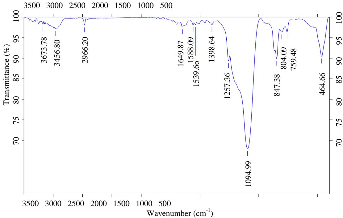
**Figure 1:** FT-IR spectra of silica aerogel powder
