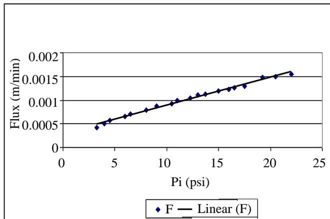
**Figure 6:** Effect of Inlet pressure on flux
