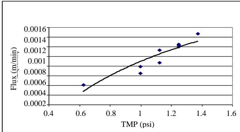
**Figure 7:** Effect of Transmembrane Pressure on Flux
