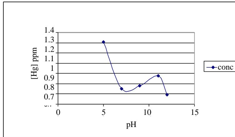
**Figure 10:** Effect of pH on Membrane without Pretreatment
