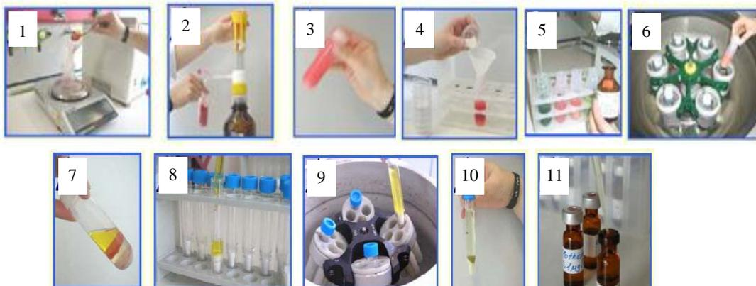
**Figure 2:** The Procedure of QuEChERS Extraction (Steven, 2010)
