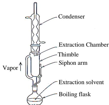
**Figure 4:** Soxhlet Extractor [14].
