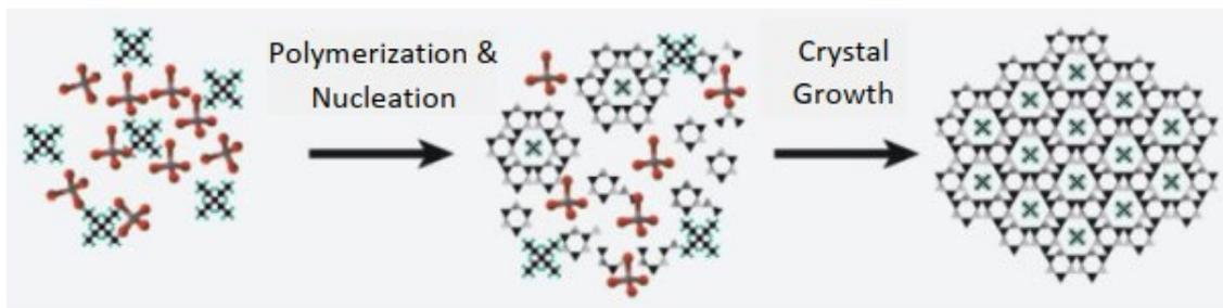
**Fig. 5** The polymerization of aluminosilicate layer to the final zeolite structure
