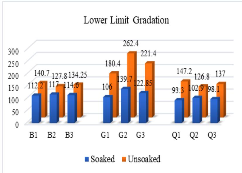
Fig. 6 - CBR value for lower limit gradation
