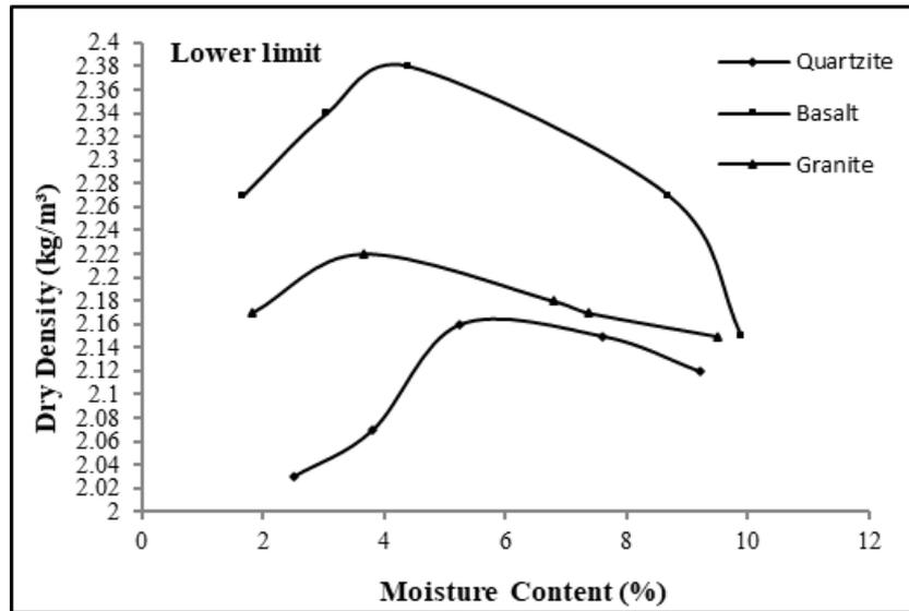
Fig. 3 - Compaction curves for lower limit gradation
