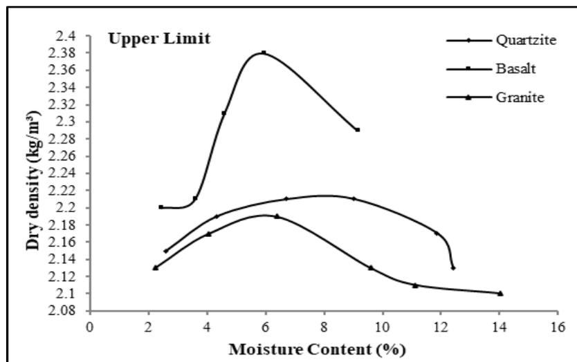
**Fig. 2 - Compaction curves for upper limit gradation**
