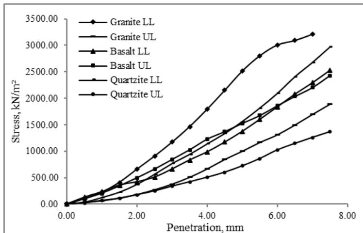
Fig. 5 - Stress versus penetration of CBR test of un-soaked samples
