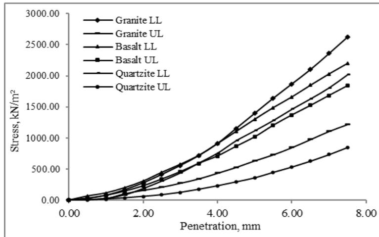
Fig. 4 - Stress versus penetration of CBR test of soaked samples
