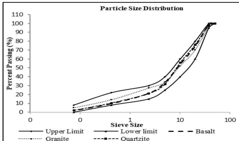
**Fig. 1 - Particle size distribution for upper and lower limit gradations**
