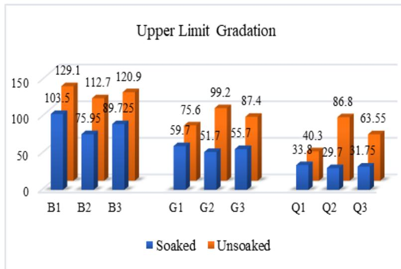
Fig. 7 - CBR value for upper limit gradation
