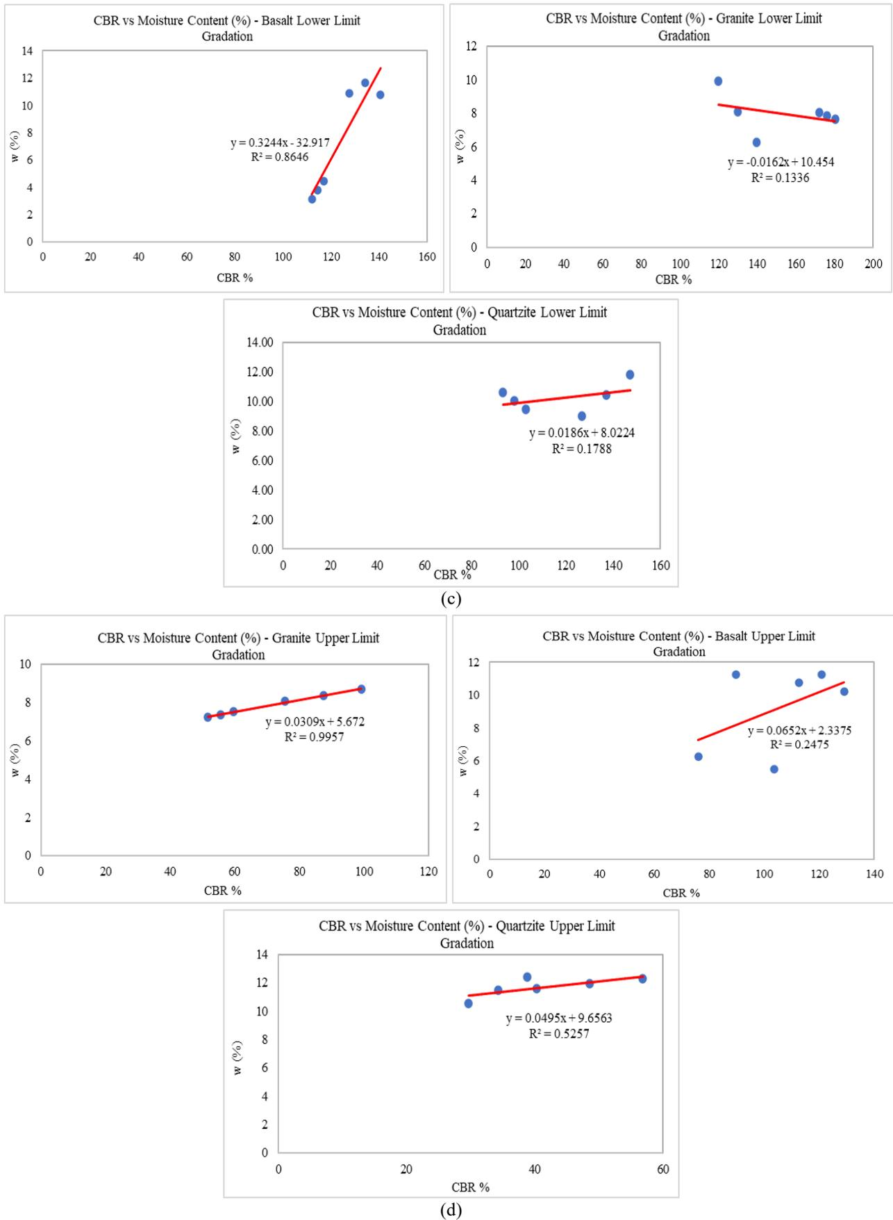
**Fig. 8 - Parameters influencing bearing ratio (CBR) values (a) materials  $\gamma_d$  for lower limit gradation; (b) materials  $\gamma_d$  for upper limit gradation; (c) materials  $w$  for lower limit gradation, and; (d) materials  $w$  for upper limit gradation**
