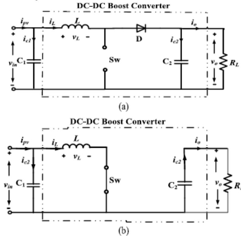
Fig. 2 DC-to-DC Boost converter operation (a) when switch is open  $u=1$ ; (b) when switch is closed  $u=0$
