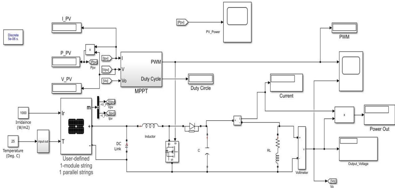
**Fig. 4 - Matlab/Simulink design model of proposed sliding mode MPPT based PV design**
