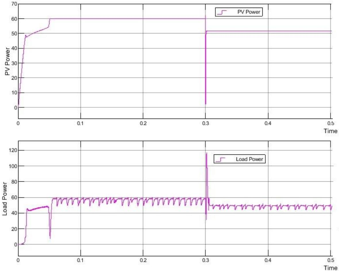
**Fig. 5 - Load and source output power variation of SISMIC design**
