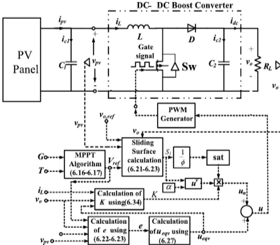
Fig. 3 SISM based MPPT design
