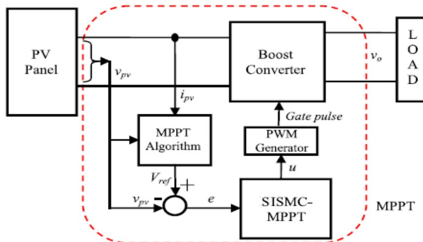
**Fig. 1 Schematic view of solar PV system model with SISM**
