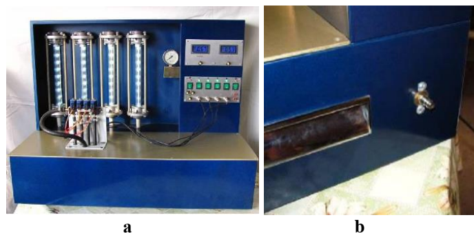
Fig. 4 - Control panel of the motorless stand (a) the general view; (b) the side view (supply of WB to the motorless stand from the drive compressor)
