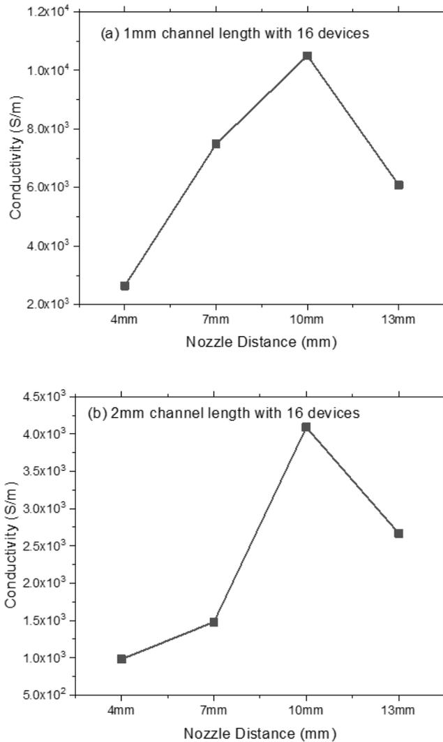
**Fig. 4 - Average conductivity at different channel length (a) 1 mm; (b) 2 mm.**
