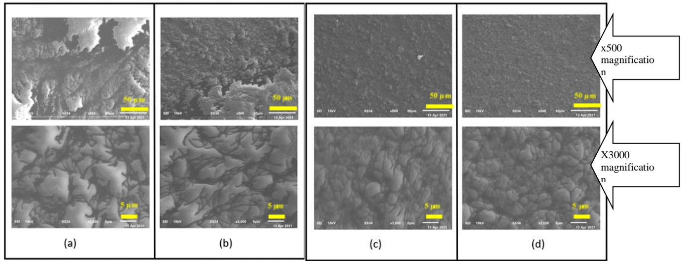
**Fig. 2 - SWCNT magnification at x500 and x3000 of CNTs spray at different nozzle distance; (a) nozzle distance of 4mm - appear glass and CNTs bundling; (b) nozzle distance 7 mm - appear glass and CNTs bundling; (c) nozzle distance 10 mm; (d) nozzle distance of 13 mm.**
