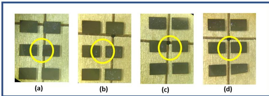
**Fig. 1 - Glass samples depositing SWCNT with 4 differences spray nozzle distance. Round circles is the location to inspect SWCNT morphology; (a) 4 mm nozzle distance; (b) 7 mm nozzle distance; (c) 10 mm nozzle distance; (d) 13 mm nozzle distance.**
