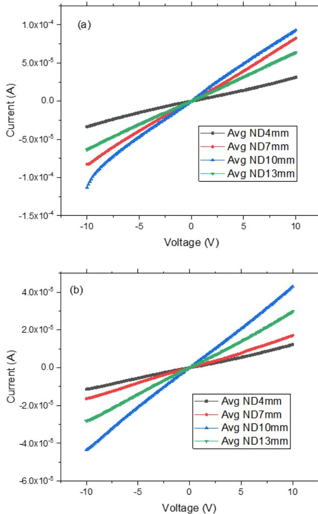
**Fig. 3 - IV plots from 32 devices from 2-terminal measurements device. It shows consistent highest current reading for 10 mm nozzle distance that reflect to morphology of SWCNT; (a) 1 mm channel devices; (b) 2 mm channel**
