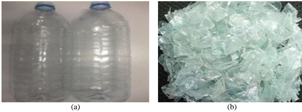
Fig. 2 - (a) Polyethylene terephthalate (PET); (b) 2.36 mm PET chips
